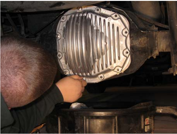
Installing the bolts after lining up the holes.
