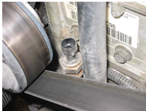
(Figure 1) Exhaust Pressure Control Valve
