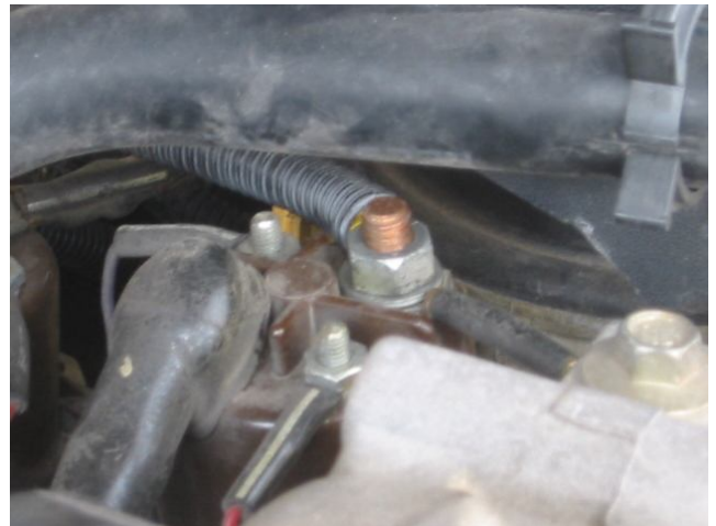
(Figure 2) Yellow Ring Bolted to Solenoid assembly
