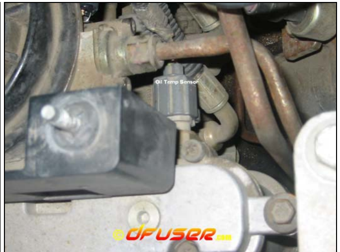
Oil Temp Sensor on Late 99-03 7.3L (Figure 10)
