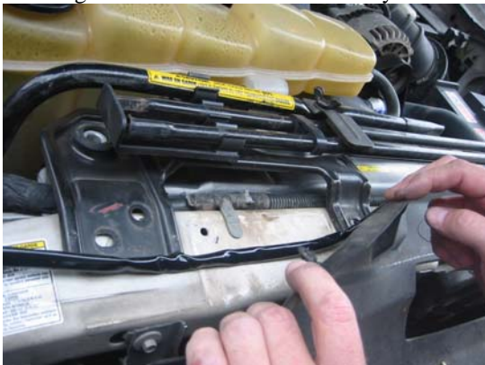
Figure 5 - Harness over the Radiator
