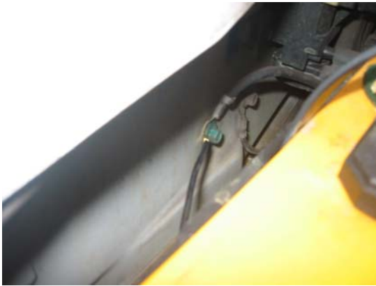
Figure 1 - Ground Passenger Side
