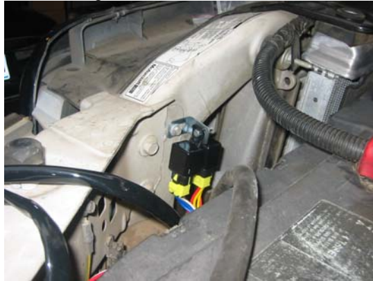
Figure 4 - Relays installed and mounted
