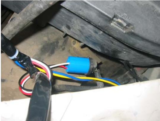
Figure 3 - Connection with Factory Harness
