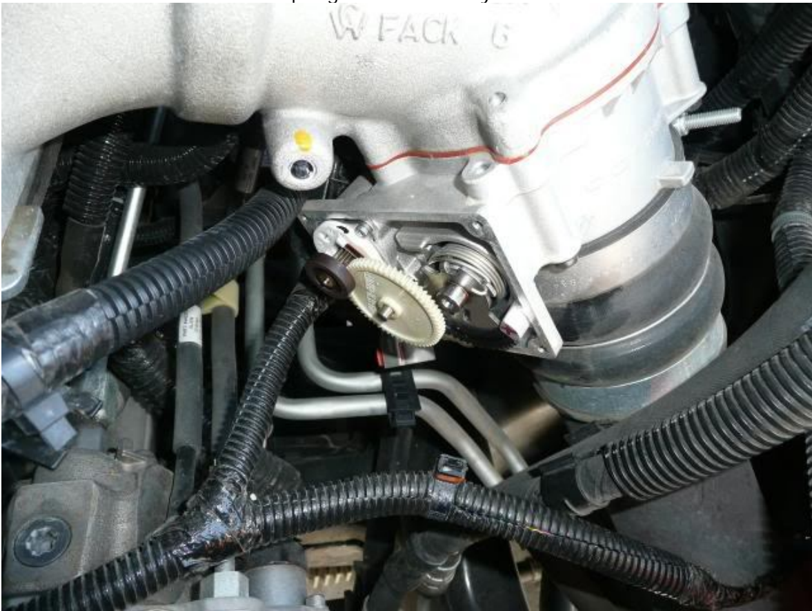
Here is the motor unit removed. NOTE the wave washer that is behind the motor. It goes back in the hole before installation of the motor again. The motor screws are T-10.
