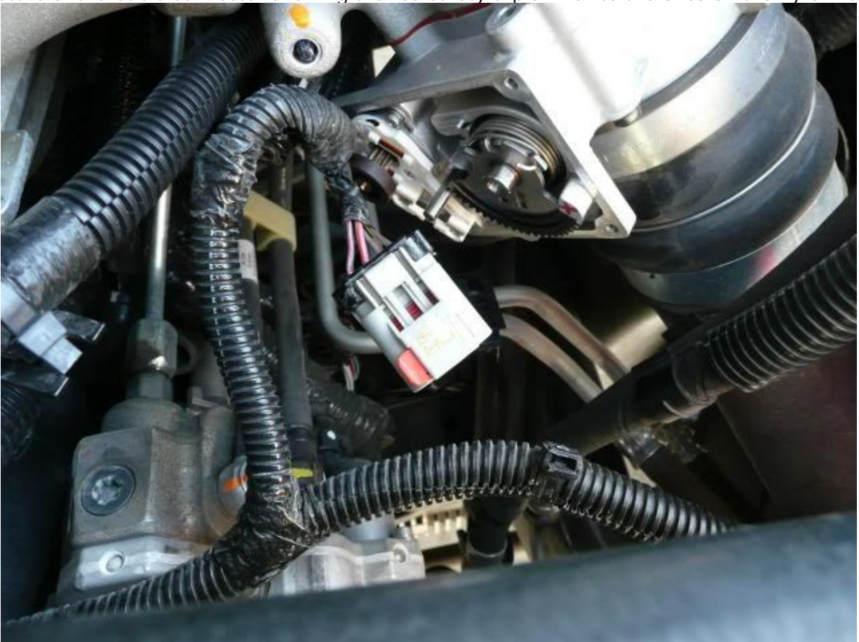
A picture of the Cable connector showing the red safety clip similar to the ones on the Pyro Probes.
